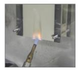
Test with a small flame: NF EN ISO 11925-2
