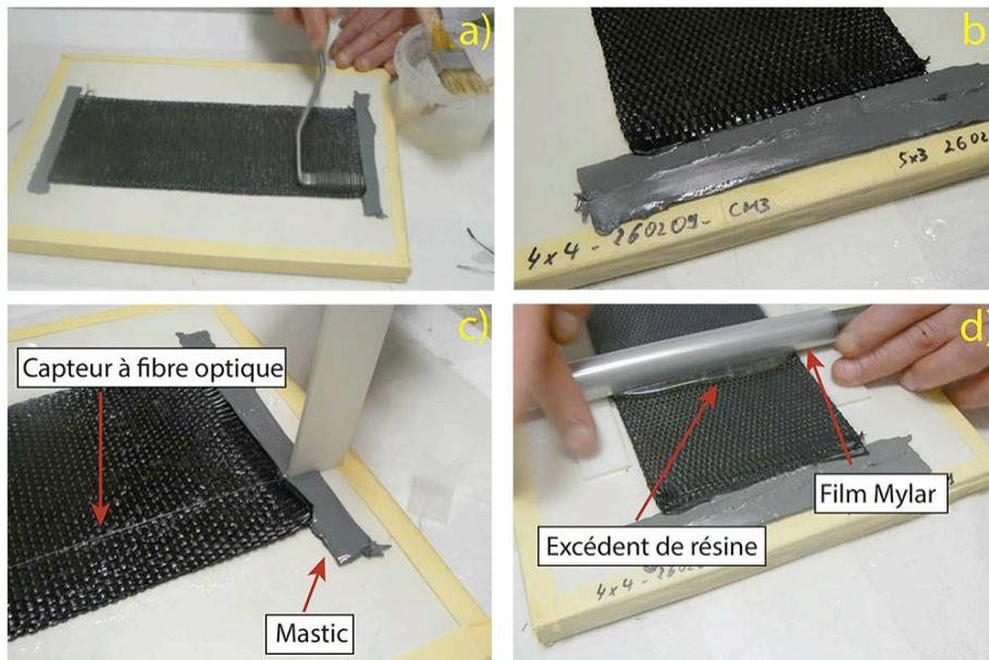
Figure 5 - The different stages of preparing a composite sample. a) Using the bubble removing roller; b) View between two layers of fabric; c) Placing the fibre optic sensor; d) Placing the Mylar film [2]
