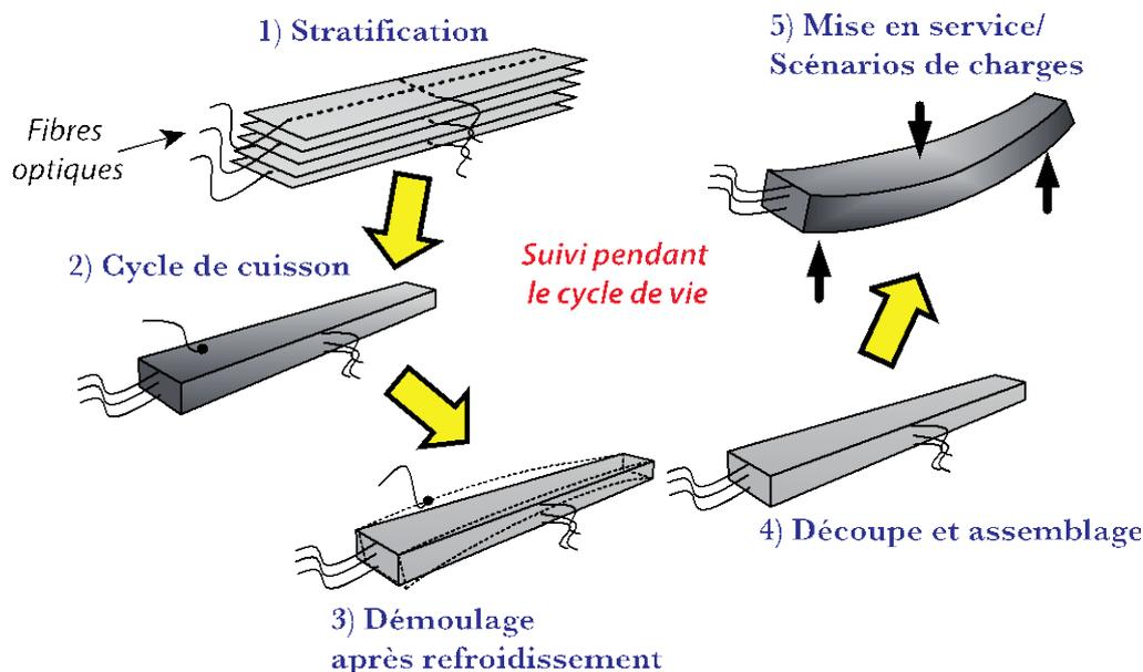
Figure 6 - Schematic diagram showing how the life cycle of a composite structure is monitored using embedded fibre optic sensors where internal deformations are monitored from when parts are manufactured until they are commissioned [5].
