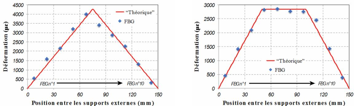
Figure 9 - On the left: Comparison between the deformation measured by the FBGs and simulated "three point" bending under a load of 633N. On the right: Comparison between the deformation measured by the FBGs and simulated "four point" bending under a load of 633N [2].
