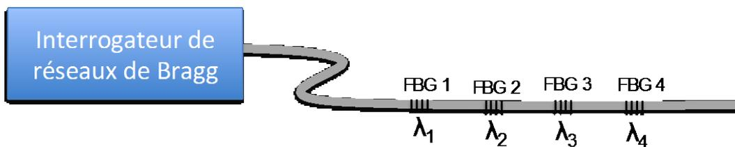
Figure 3 - Wavelength multiplexing with Fibre Bragg Grating sensors
