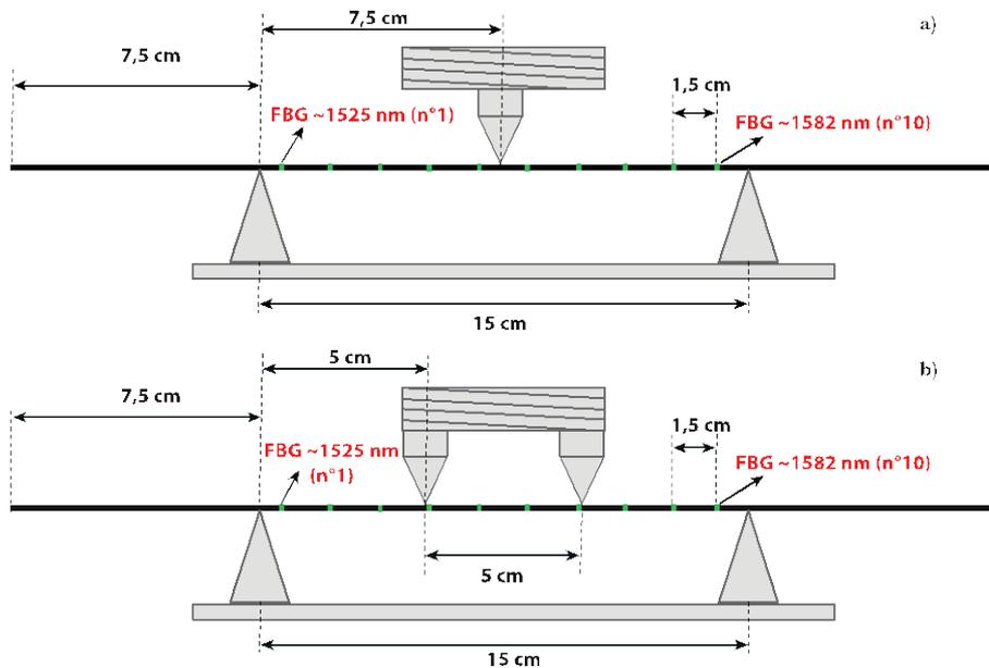
Figure 8 - Diagram of an (a) three point and (b) four point bending test with the position of the sensors embedded in the composite in relation to the support points [2]
