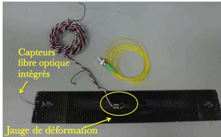
Figure 4 - Comparison between a strain gauge and an optical fibre comprising several Bragg gratings [2]
