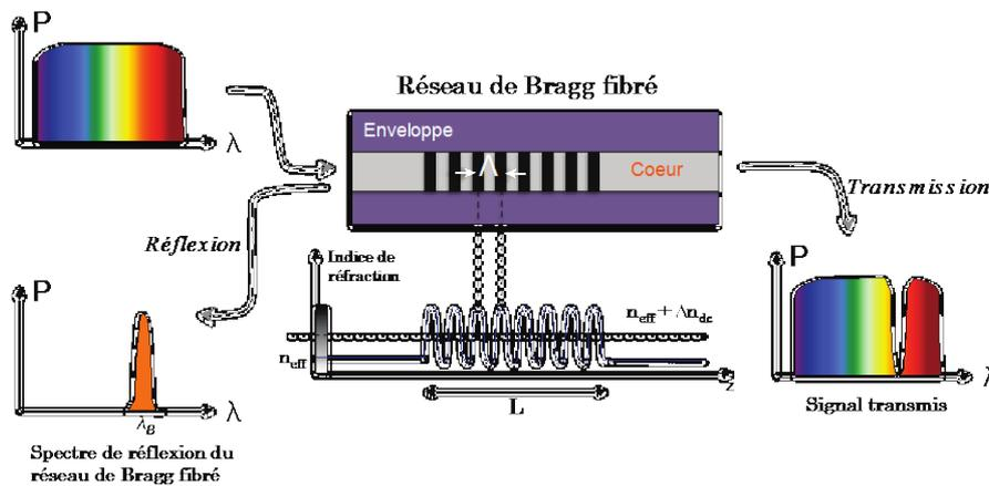
Figure 1 - Fibre Bragg Grating and spectral effects
