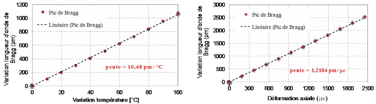
Figure 2 - On the left: Change in Bragg wavelength depending on temperature. On the right: Change in Bragg wavelength depending on deformation [2]
