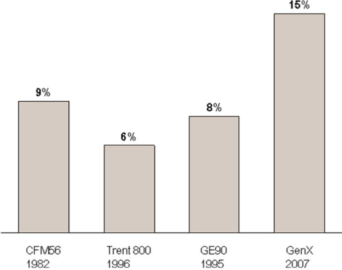
Figure 10: Level of composites in aircraft engines<sup>12</sup>
