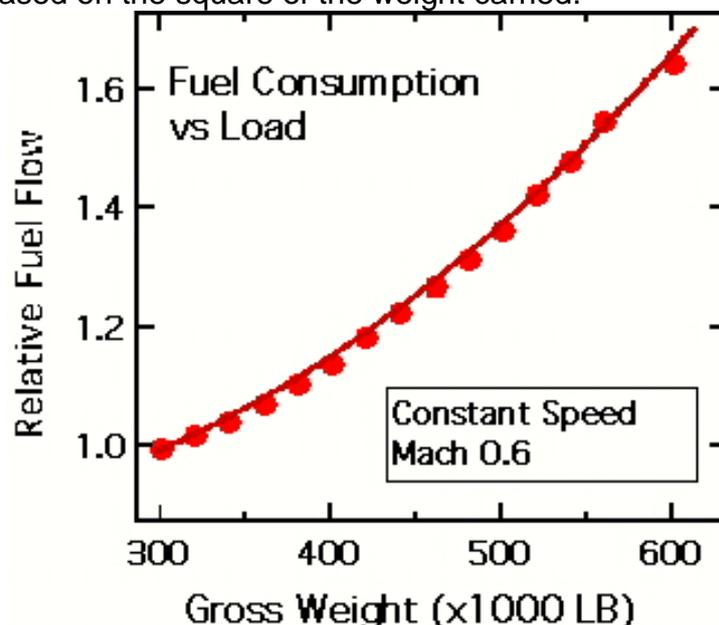
Figure 1: Fuel consumption according to load for a large transport aircraft flying at constant speed.<sup>1</sup>
