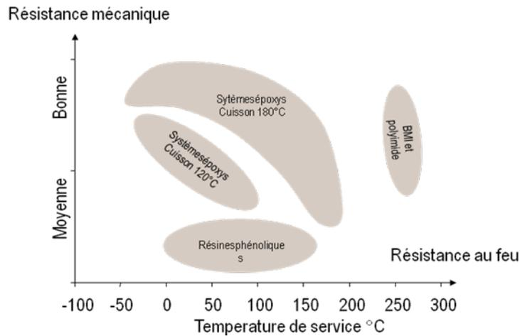
Figure 11: Types of thermosetting resins used in aeronautics<sup>13</sup>
