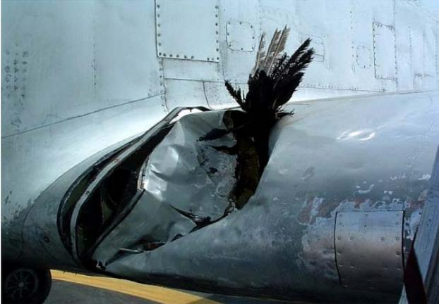
Figure 4: Impact of a bird on the wing of a plane with a metal structure.
