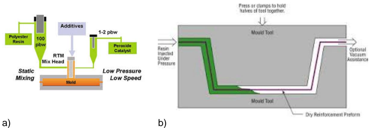
Figure 14: RTM: a) installation diagram b) principle
