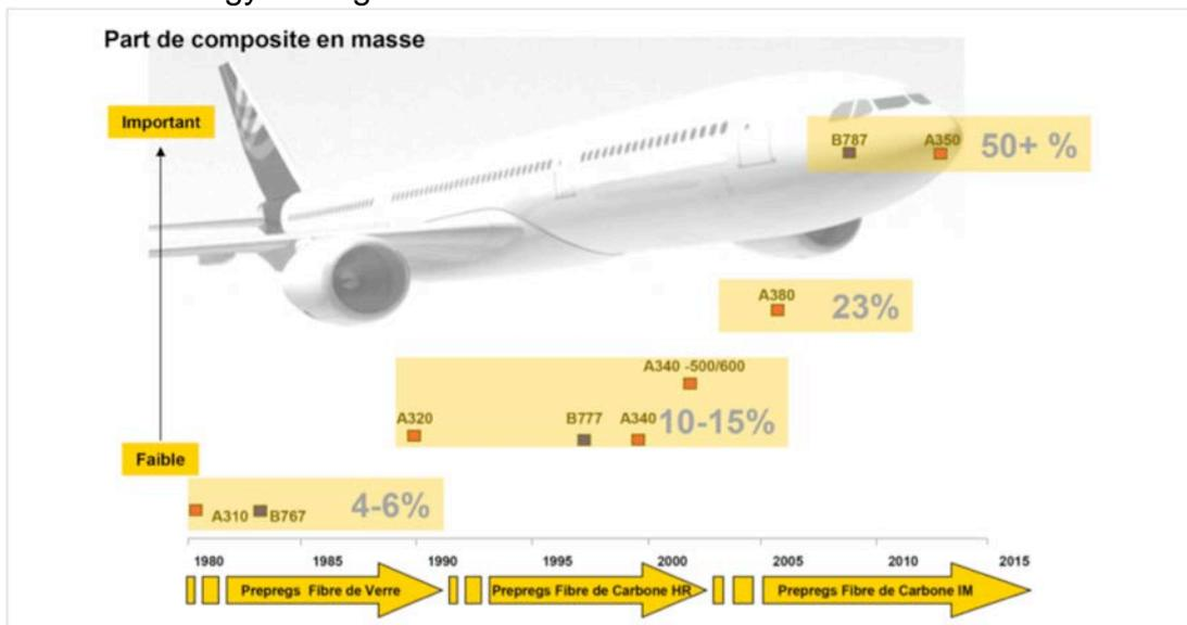
Figure 3: Share of composites in the structure of modern civil aircraft.<sup>3</sup>
