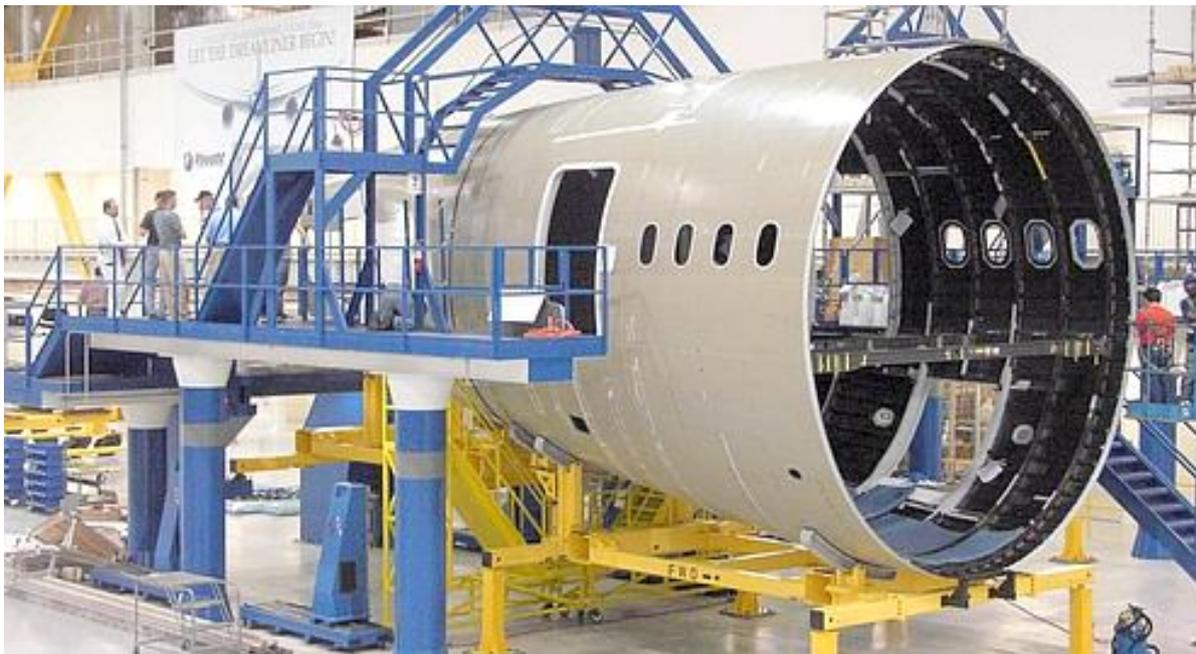
Figure 7: Part of the fuselage of the Boeing 787 Dreamliner
