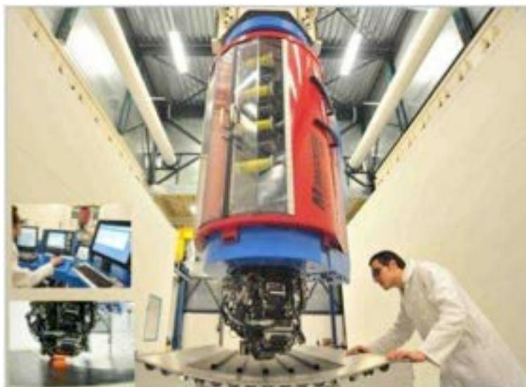
Figure 12: Automated Fibre Placement (AFP) (doc. Sonaca)
