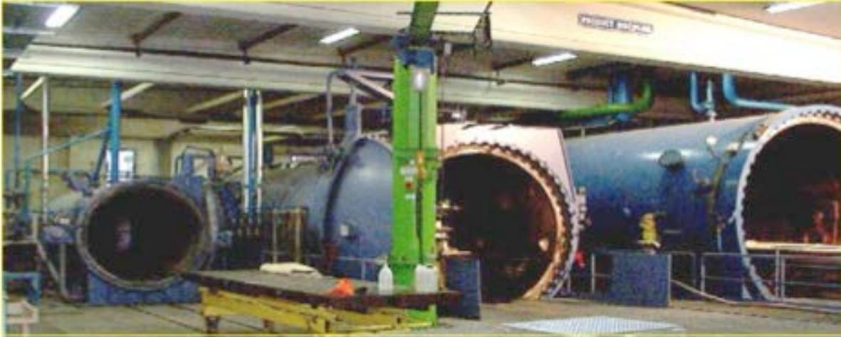
Figure 13: Autoclaves used for aircraft parts (doc. Sonaca)
